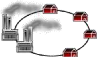
Loop feed with multiple power sources and paths
