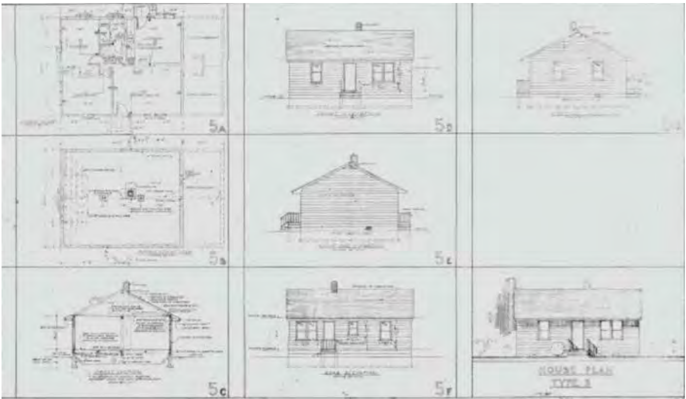
Figure 52 : Government blueprints for 'Indian House type 5' from the 1960s — one of the designs used for reserve housing. Source: Library and Archives Canada.
