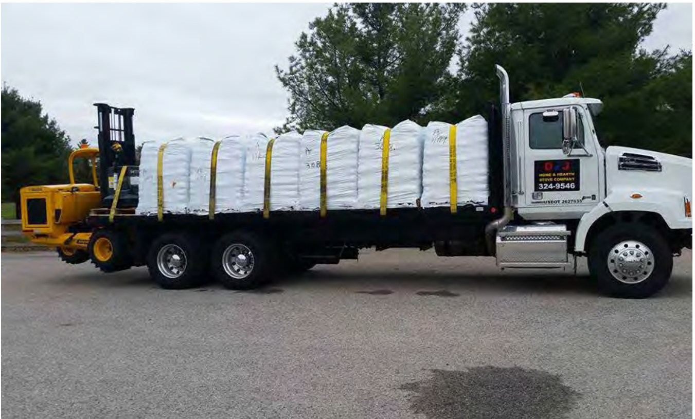
Figure 91 : wood pellet delivery using flatbed truck and forklift. Source: www.woodpellets.com
